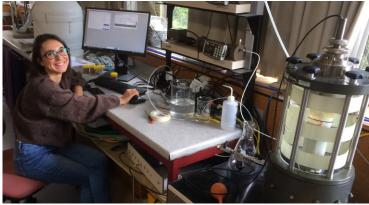
Jordanka conducting triaxial tests. The triaxial apparatus (on the right) puts controlled stress on our tephra samples so we can study their response. This helps us relate the liquefaction within the tephras to past earthquakes.
